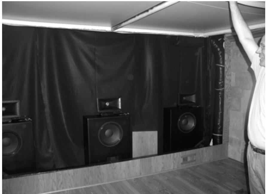
Figure 12-6. Front loudspeaker array, left, center and right shown with the screen lifted out of the way. Note black absorb- ing material on back wall for both sound and light.
