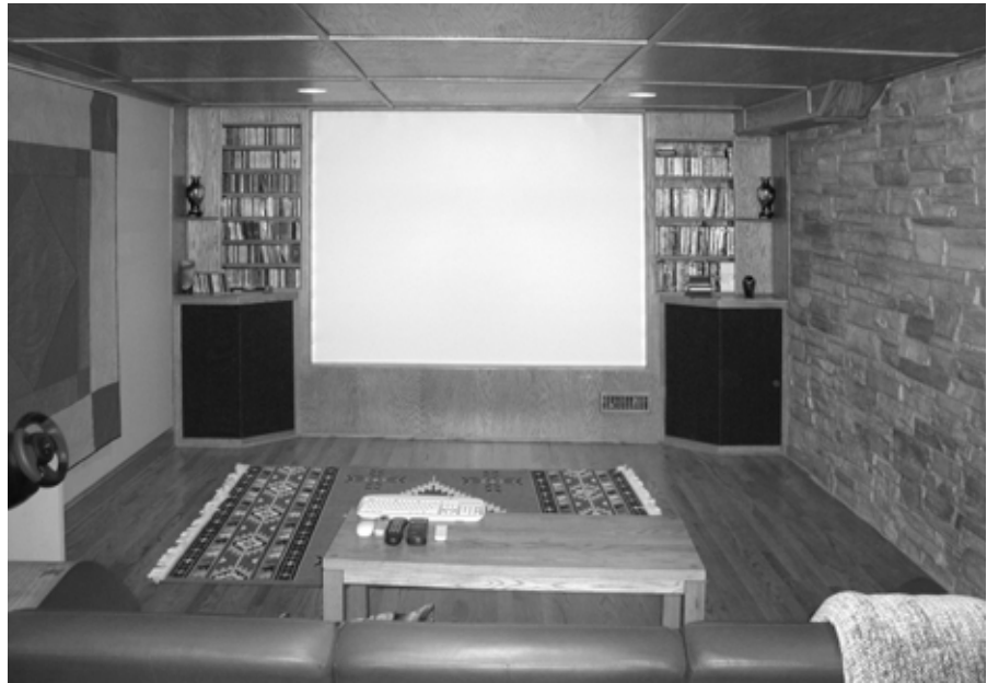
Figure 12-8. The authors HT looking towards the screen. This is a 4:3 setup 1024x768, DLP projector. Note cultured stone wall on right and (light) sound absorbing wall quilt on the left. ALSO on the left is the game wheel for a driving simulator. The speakers are behind the black grills. Plans are to convert this setup to 16:9.
