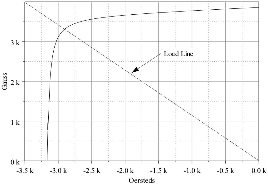
Figure 2-5 - Ceramic magnet load line calculation - the dotted line is the load line
