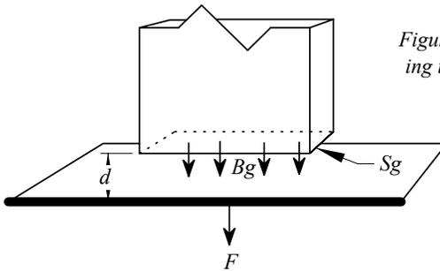
Figure 2-3 - Tractive air gap showing the variables used in the equa-
