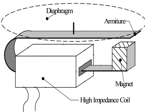
Figure 2-2 - Variable reluctance motor structure
