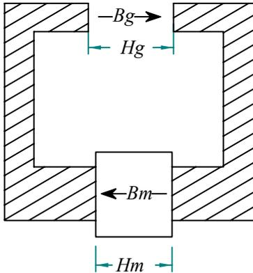
Figure 2-4 - Magnetic circuit definitions
