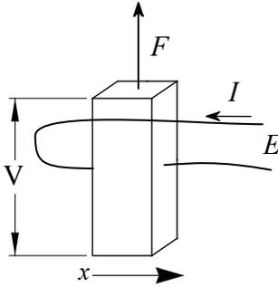
Figure 2-6 - Diagram of piezoelectric X-cut crystal actuator
