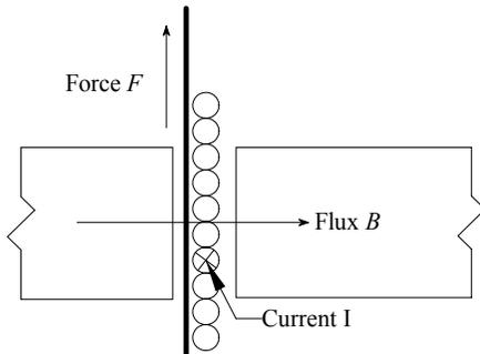
*Figure 2-1 - Moving coil topology with definitions*
